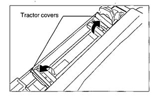
6 Align the paper sprocket holes with the tractor pins, then close the tractor cover.
