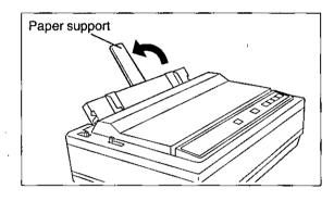
**11** Insert the paper support into the slot of the extension plate until it stops.
