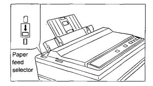
**5** Press **LOAD/PARK** to reload the fanfold paper to the first print line.
